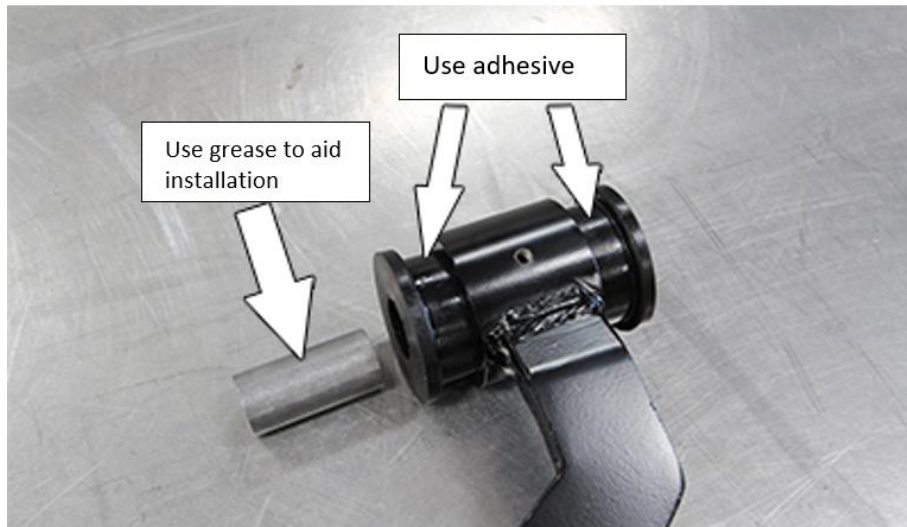
Figure 3: brushing and crush sleeve installation
