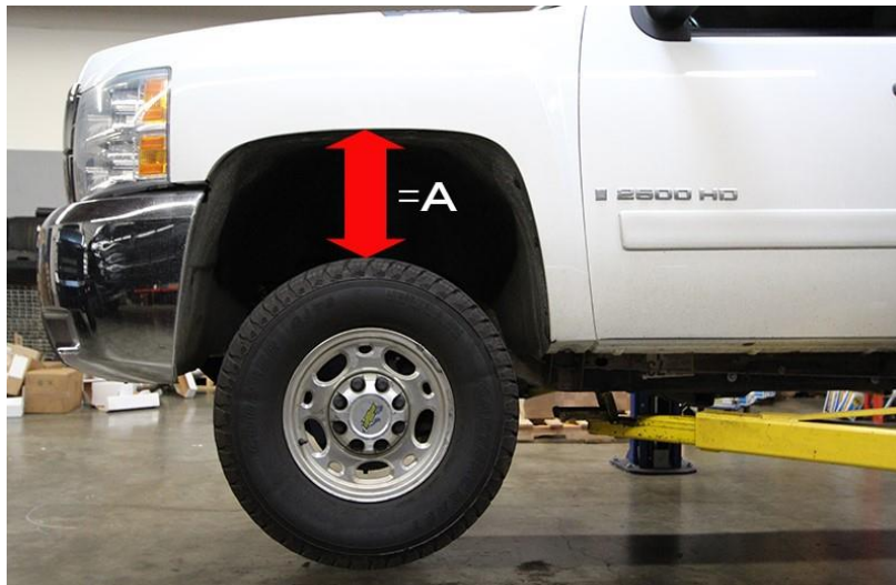
Figure 5: Distance between top of tire and fender lip
