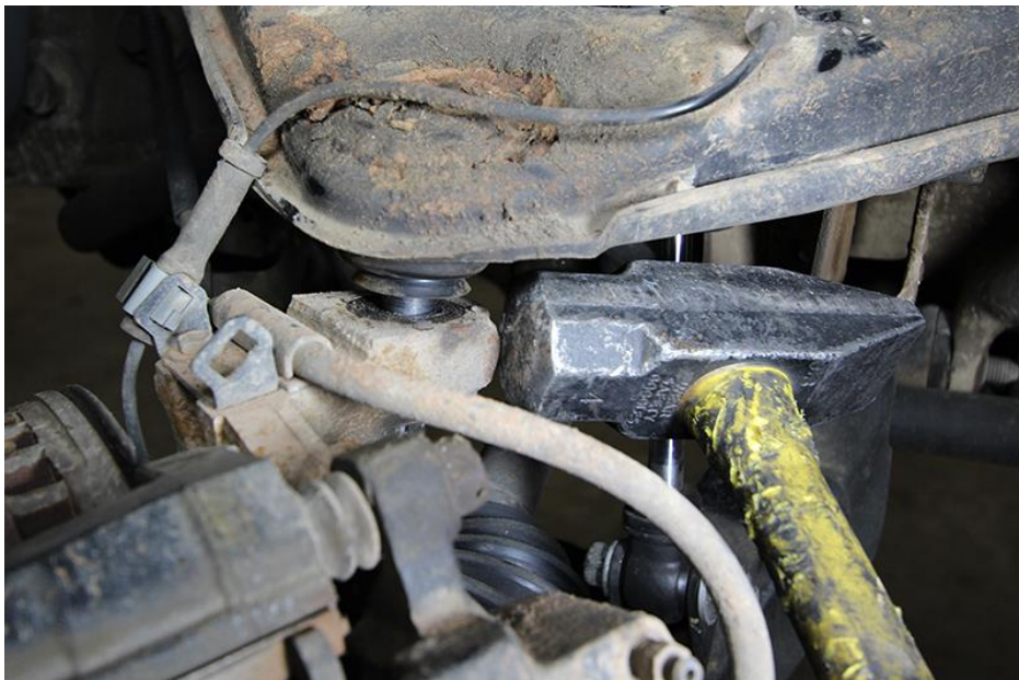
Figure 1: breaking ball joint loose from spindle
