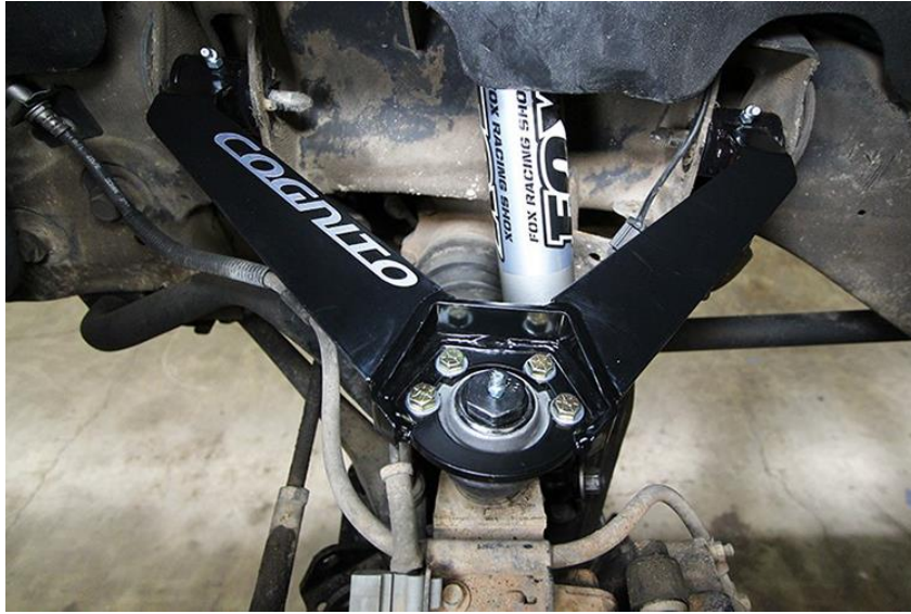
Figure 4: Driver side Cognito control arm installed
