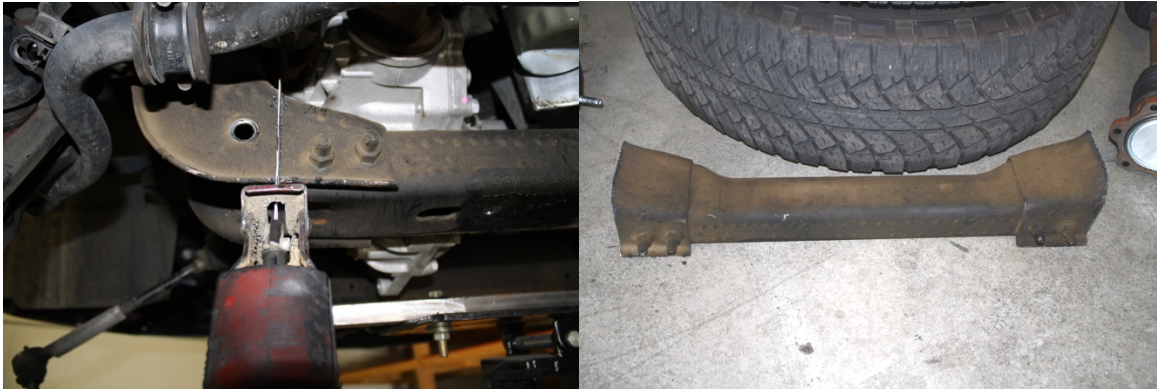
Figure 6 & 7: cut & removal required to make room for the repositioned differential.
