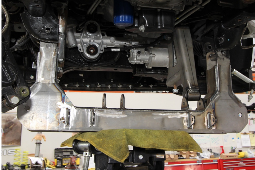
Figure 12: bolt in rear crossmember.
