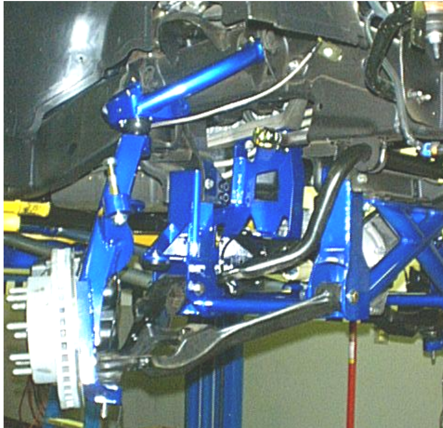
Figure 8. Spindle assembly and lower control arms installed.
