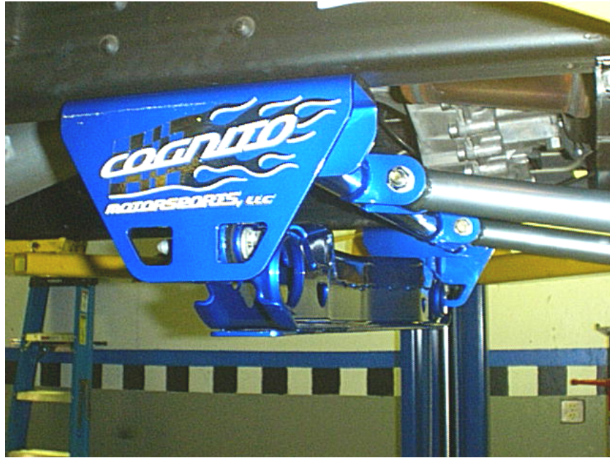
Figure 10. Torsion bar drop mounted to compression struts, and to the bottom of the frame rails.
