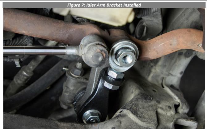
7. Tighten the idler pivot nut to 85 Ft.-lbs. before reinstalling the idler pivot into it's frame mounting pocket. Reinstall the two bolts and tighten to 78 Ft.-lbs.
