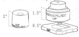
Recommended Bump Stop configuration based on tested tires. Not all Tires Measure the Same. Cycling the suspension to check the shocks, springs and other suspension componets before driving is recommended.
