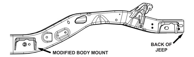
CUT OUT THE TEMPLATE AND PLACE IT ONTO THE REAR BODY MOUNT
