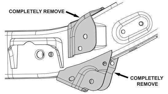
COVER ANY FUEL LINES WITH WET RAGS AND MOVE ANY WIRES OR LINES BEFORE CUTTING THE BRACKETS OFF
