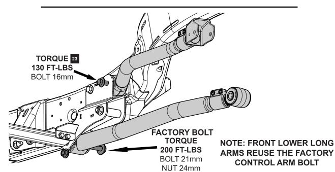
IF INSTALLING LONG ARMS WITH IR BUSHINGS YOU CAN TORQUE THE ARM BOLTS NOW, OTHERWISE WAIT UNTIL THE JEEP IS ON THE GROUND
