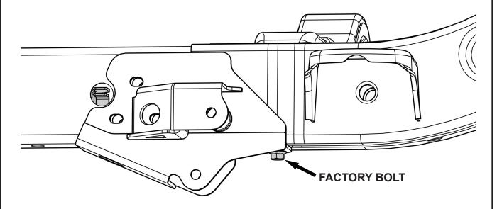
USING THE FACTORY BOLT TO HOLD THE BRACKET TO THE FRAME, SLIDE THE TWO FLAG NUT ASSEMBLIES INTO THE FRAME AS SHOWN IN STEPS 57-58
