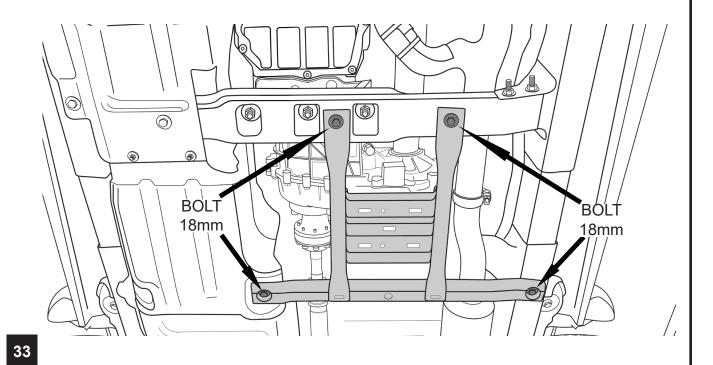
DISCONNECT THE FUEL LINES AND REMOVE THE FRONT SECTION OF THE GAS TANK SKID PLATE
