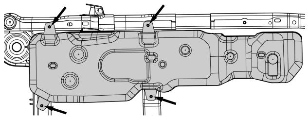
REMOVE THE 4 18mm BOLTS AND LOWER THE GAS TANK UNTIL YOU HAVE ENOUGH ROOM TO DISCONNECT ALL FUEL AND ELECTRICAL LINES FROM THE TANK
