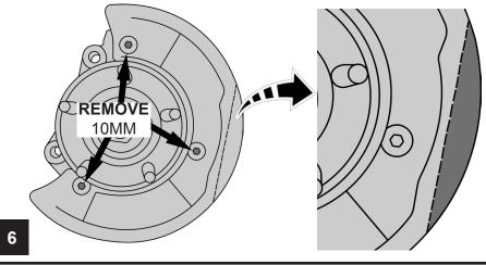
ONCE REMOVED FROM THE AXLE, GENTLY BEND THE FRONT EDGE INWARDS AT THE INDENTED LINE.
