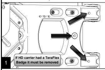
Position the mount and start the M8 bolt(7) and washer(8) into the mounts upper left hole, spacer(10) will go between the mount and carrier, leave bolt loose. Note: If there is a problems starting the M8 bolt, test fit spacer and bolt, without mount, to move nut into position. Next tighten the left bolt to keep plate in position, then remove spacer and M8 bolt, install as before.
