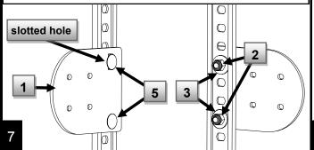
The RotopaX Mount can also be mounted directly to the Hi-Lift Mount by installing two 1/2 x 1.25" carriage bolts(4) through the RotopaX Mounts square holes and Hi-Lift Mount top two outer most holes. Each bolt gets a washer(3) and nut(2). Tighten nuts to 55 ft-lbs.
