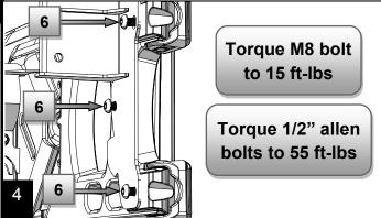
Have Hi-Lift Jack completely collapsed before installing. Push Hi-Lift Jack onto the bolts, adjust the top bolts position in slotted hole to best line up holes in the jack. Start 1/2" washers(3) and nuts(5) onto the 1/2" bolts(4), **do not tighten nuts.** With the top bolt lined up with the Hi-Lift Jack holes torque the top bolt to spacer (65 ft-lbs). Tighten both 1/2" nuts(5), securing the jack, then carefully check that the base of the jack will clear the body when the tailgate is fully open.
