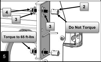
Using a 12mm socket remove the upper right M8 bolt that fastens the HD Hinged Carrier to the tailgate and loosen the other M8 bolt that is just to the left it. Note: These two bolts use the same floating captured nut plate inside the tailgate. By loosening the left bolt the plate will allow for better fitment.
