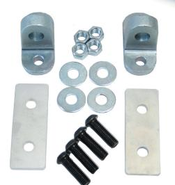
Place D-ring mounts on the front of the TJ front bumper using the bolts provided. Bolt them to the bumper using the pre-drilled holes. Place backing plates on the inside of the bumper sliding them onto the backside of the bolts holding the D-ring followed by the washer and nuts.
