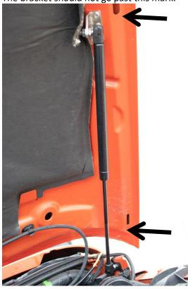
Place the very edge of the mounting bracket on this line, and mark the location of the three holes.
