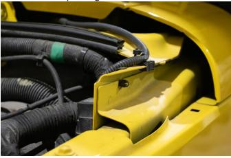
With a 5/16" drill bit, drill out this hole on each side.
