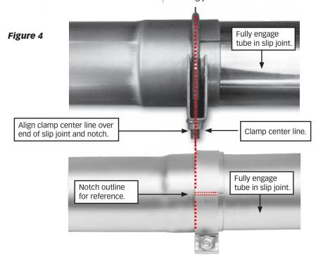
**12.** Install Banks Monster tailpipe tip with exhaust band clamp on the exhaust. Keep the wrapping on until installation is complete.
