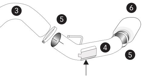
Note: Clearance between heat shield and spare tire must be greater than 1/4 inch. This clearance can be increased by shifting the spare tire further from the exhaust.
