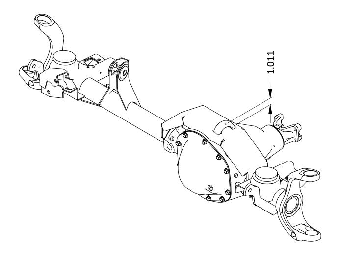
Step 6: Weld 2 posts into cut outs.
