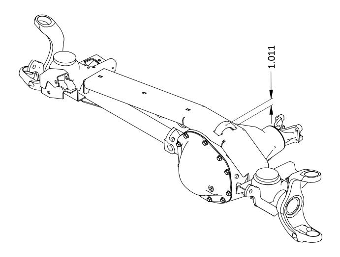
Step 8: Make 5 1" welds along gusset to axle tube on both sides.
