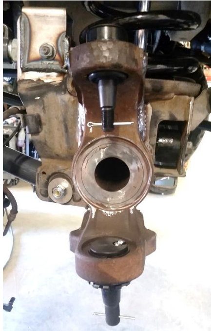
Figure 13. Cotter Pins Aligned Front to Back
