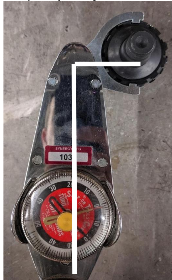
Figure 20. Incorrect Wrench Orientation
