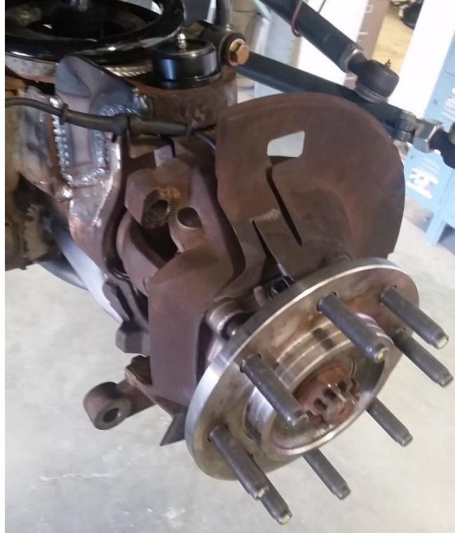
Figure 16. Backing Plates, Hubs and ABS Lines Re-Installed
