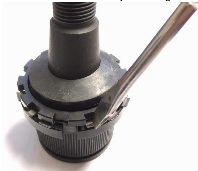
Figure 18. Bending Locking Tabs Back
