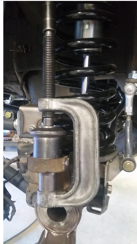
Figure 8. Pressing Out Lower Ball Joint Figure 9. Pressing Out Upper Ball Joint
