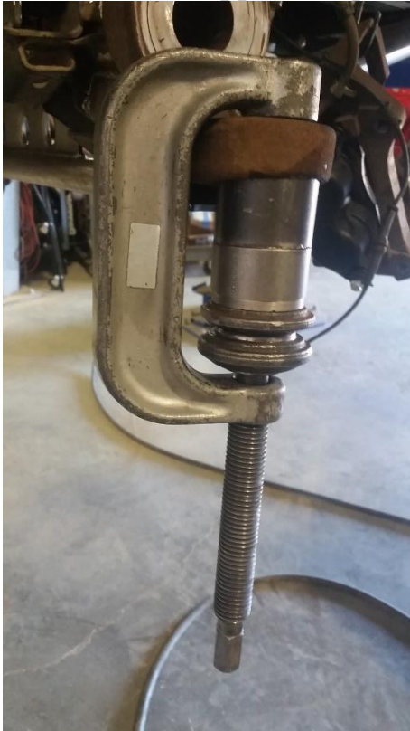
Figure 8. Pressing Out Lower Ball Joint Figure 9. Pressing Out Upper Ball Joint
