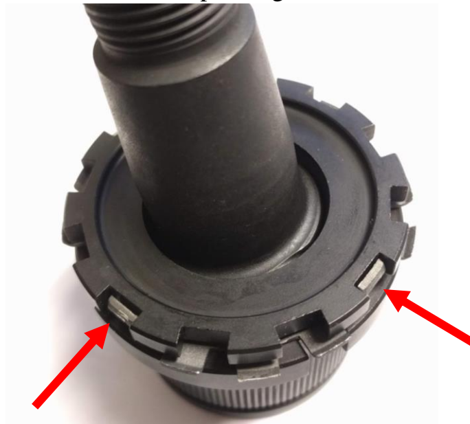
Figure 15. Tabs Bent Into Cap
