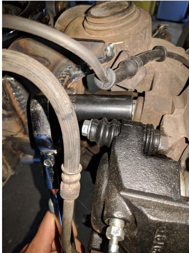
Figure 2. Removing Brake Caliper Carrier Bolts
