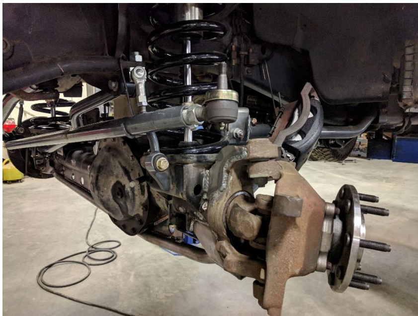
Figure 4. Tie Rod Removed
