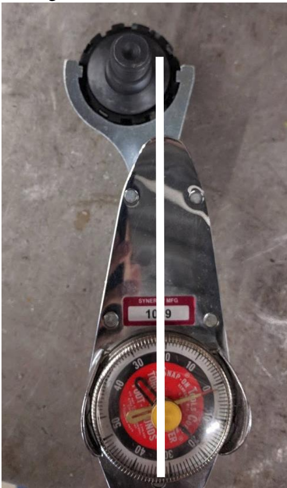
Figure 19. Correct Wrench Orientation
