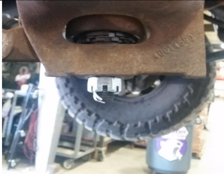
Figure 14. Cotter Pin Installed
