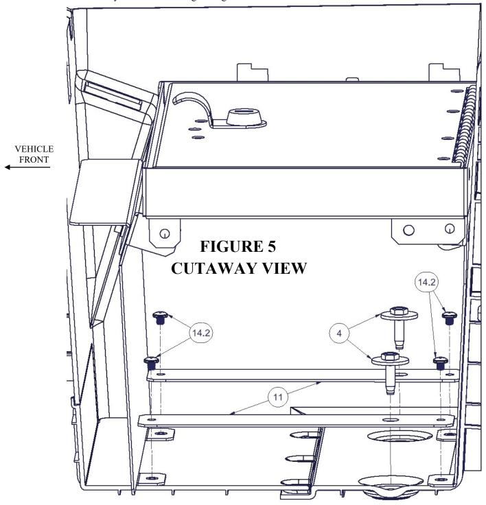
13. Reinstall the (2) #4 Console Mounting Bolts (removed in Step 6) in the factory locations and tighten to about 4 ft-lbs, or until the bottom of the #11 Plates meet the bottom surface of the console in the area around the concave inset.
