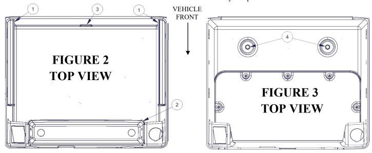
7. Using a 10mm socket remove the (2) #4 Factory Console Mounting Bolts shown in Figure 3.
