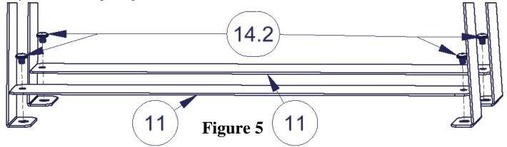
9. Replace contents of console, the pad removed in Step 3 will cover the bottom plates and their associated hardware. The factory coin tray may be utilized or removed depending on your preference.
