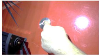
With the other, secure a washer and a nut to the countersunk bolt. With a 13mm socket and 5mm allen key, tighten the nut and repeat on the opposite side.
