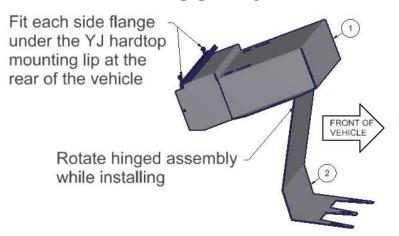
6. Position the Hinged Panel assembly #1 & #2 in the vehicle and align the obround holes in the mounting flange with the (3) rear seat belt bracket holes, as illustrated. Re-Install the #5.4 bolts and #5.8 seat belt brackets in their original locations. Do not tighten bolts at this time. (Figure 4)
